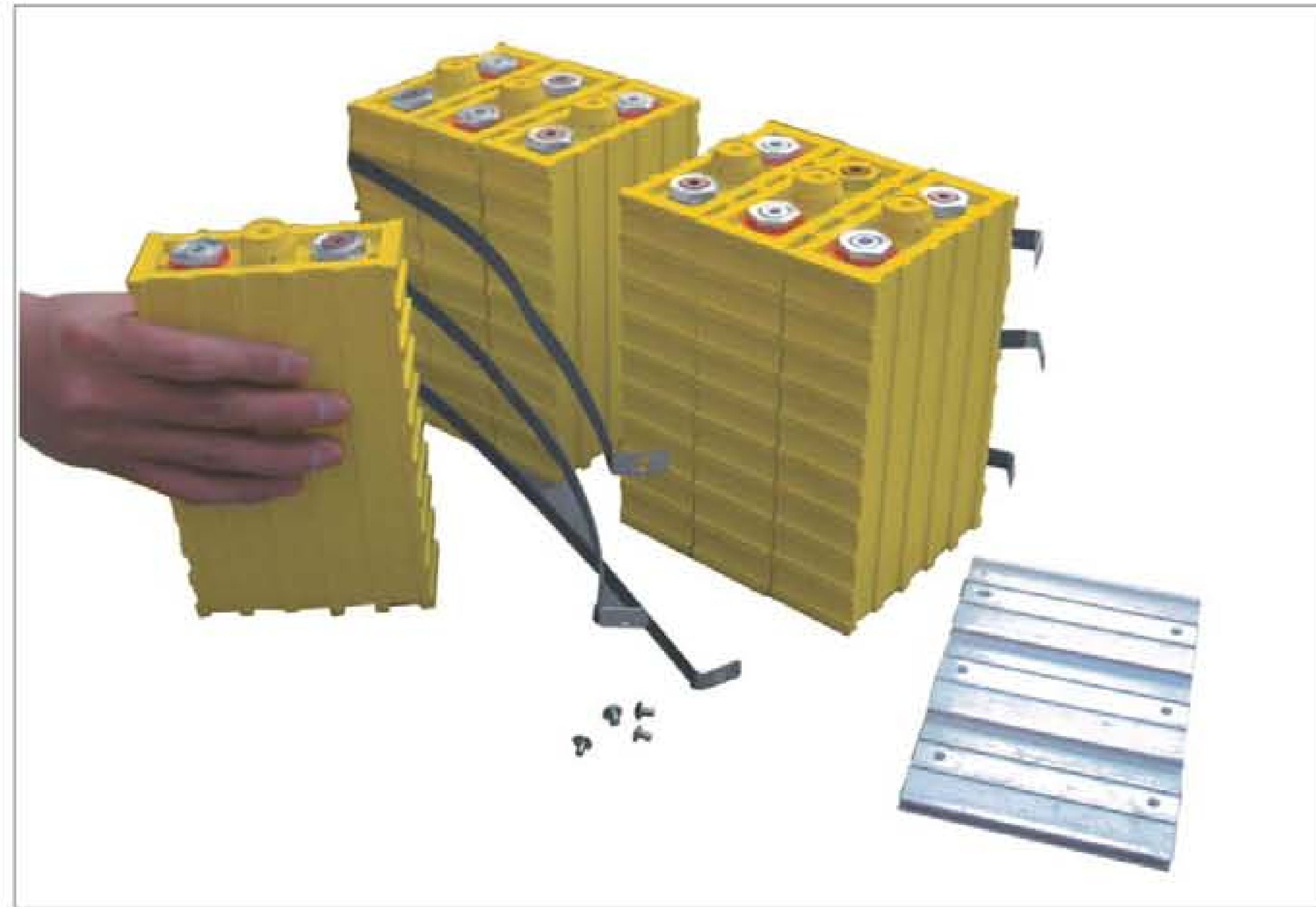
Release the strap and replace the cell with same capacity.
