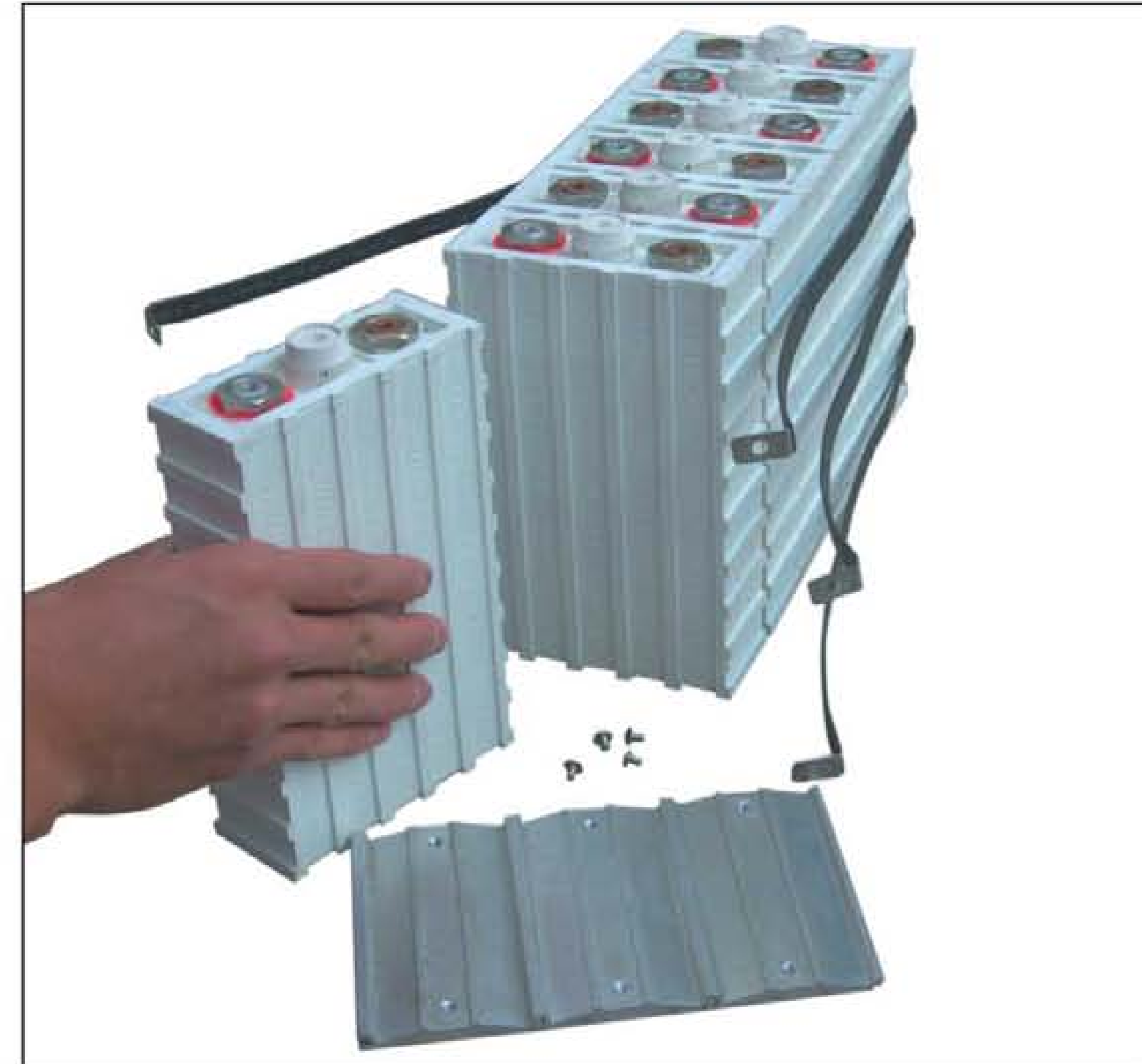
② Release the straps and take out the cell you need to replace
